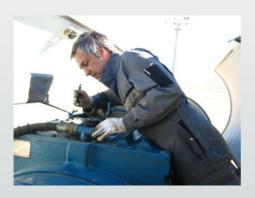
Inspection of gearboxes through available inspection apertures
